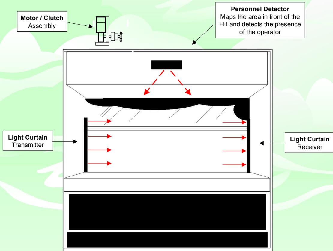
The Green Sash System auto Sash Closer for Fume Hoods is primarily designed for operation on Fume Hoods with VAV controls and has the following features and benefits :-
