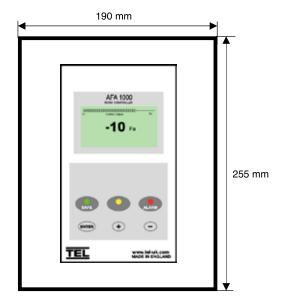
Enclosure Dimensions Enclosure with hinged lid (hinges on the left hand side) Cable knock outs 3 x M20 Top 3 x M20 Bottom
